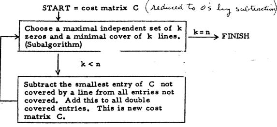
FINISH = maximal independent set of n zeros determines optimal assignment for cost matrix C.
